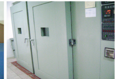
Temperature cycling test chamber
